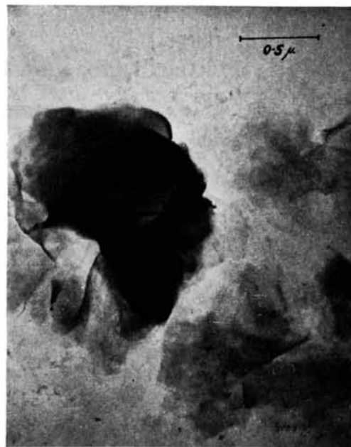
Fig. 2. Electron micrograph of montmorillonite particles, showing thin portions, and a much thicker aggregate.
